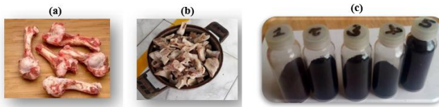
Figure 2: The images of VNBC synthesis process in laboratory. It is denoted that Figure (a) as bovine bones collected from cow slaughterhouse, Figure (b) as bovine bones collected from cooking shop of noodle soup with beef, and Figure (c) as bovine bones synthesized to VNBC, respectively.
