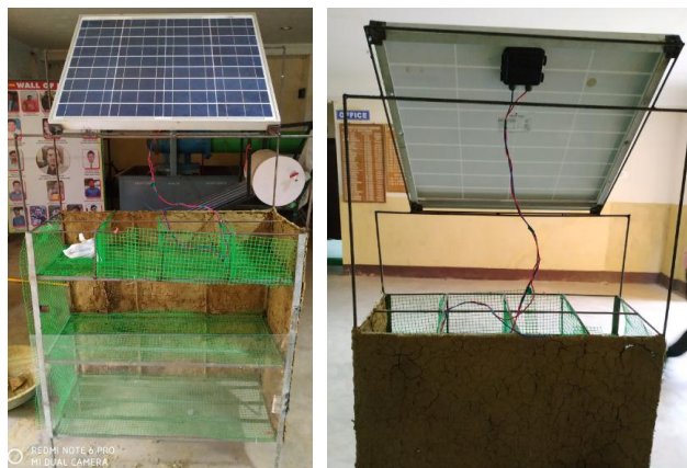
Fig-1: Skeleton Model of Scientific development of Mansukh Bhai's Mitti Cool Refrigeration System
