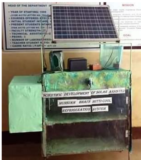
Fig 5: Final prototype of Scientific Development of Mansukh Bhai's Mitti Cool Refrigeration System
