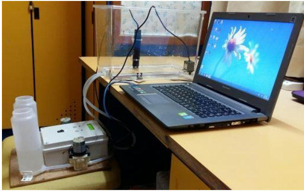
Figure 6: Experiment Setup for Automated pH Regulator For Freshwater Prawn with pH Meter Pro
